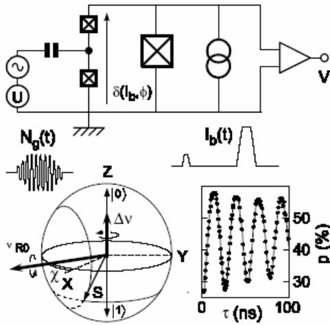
Fig 1: top: circuit diagram of the qnantronium. The Hamiltonian is controlled by two parameters: the charge coupled to the box island between the two small junctions, and the phase across their series combination. The qubit state is manipulated by applying resonant microwave pulses, or adiabatic pulses on the control parameters. The oscillations of the switching probability of the readout junction reveal the Rabi oscillations of the qubit state.
