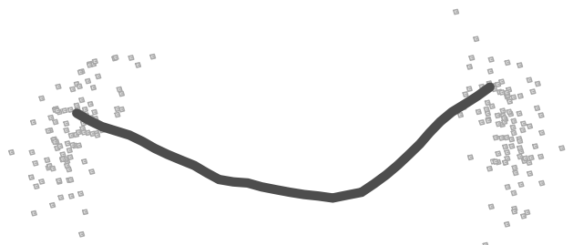
FIG. 1. Cloud of end points generated by simulating N = 100 realizations of the dynamics starting from the illustrated initial condition. The moments of this cloud are used to distinguish the longitudinal and transverse dynamics. The transverse fluctuations are larger in amplitude than the longitudinal fluctuations.
