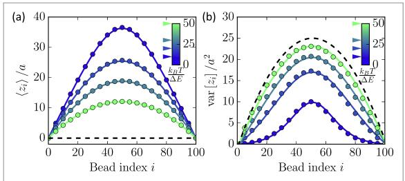
**Figure 2.** Stationary state statistics of the loop. Mean (a) and variance (b) of the position of beads in the one-dimensional pinned polymer loop from Monte Carlo simulation results (dots) are compared to theoretical results (solid lines). The number of beads in the polymer loop is L = 100. The dashed line indicates the case of no external force  $k_B T/\Delta E \to \infty$ . Other values of  $k_B T/\Delta E$  are shown by different colors as indicated in the legend.
