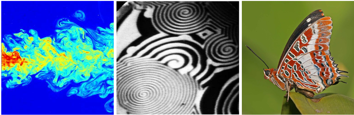
Figure 1.5: Examples of pattern formation in complex systems. Left (A): Turbulent flow in water visualized using laser-induced fluorescence [123]. Here the field of view is 45 \times 45 \text{ mm}^2 . The false-colour scheme represents the concentration of a fluorescent dye, with red representing the highest concentration and blue the lowest. Image reproduced with the permission of J. Westerweel. Center (B): Spiral patterns in the oxidation of carbon-monoxide on platinum revealed via photoemission electron microscopy [124, 125]. Here dark regions are covered in oxygen, and bright areas are covered in carbon-monoxide. The dimensions of the image are approximately 445 \times 410 \mu\text{m}^2 . Image reproduced with the permission of G. Ertl. Right (C): Pattern formation in a butterfly wing. Photograph used with permission from the photographer, Muhammad Mahdi Karim [126]. Images from panels (A) and (C) appeared on Wikipedia in addition to the given original citations [127].
