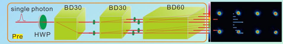
Pre: State preparation HWP: Half Wave Plate BD: Beam Displacer 30 or 60 mm
