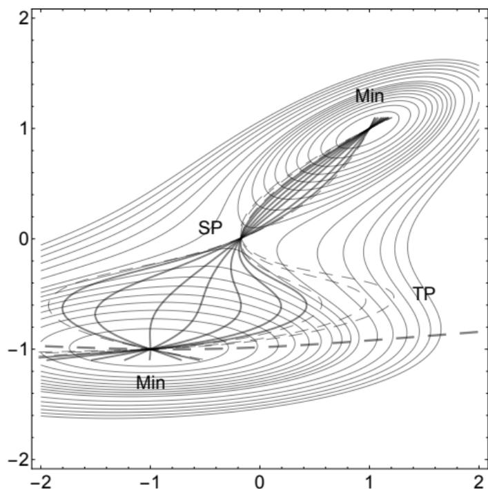
Pulling into a defined direction uses a respective NT for the movement of minimum and SP. The arc of the NT can be of different length. Thin dashed NTs have a turning point (TP): pulling along such NTs is possible.
