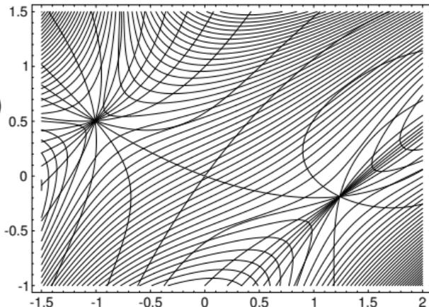
Two consecutive saddles can be connected only by a singular Newton trajectory which crosses a valley-ridge inflection (VRI) point.
