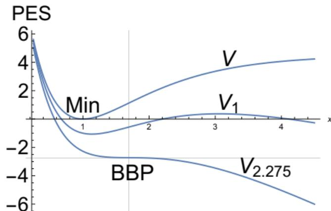
1D Morse potential over the  $x$ -axis: the upper curve. Below are two effective potential curves with increasing forces. The minimum moves to increasing  $x$ -values, where the SP moves to decreasing values. The lowest potential is the final case: minimum and SP coalesce to a shoulder. The former barrier is broken. The point is named barrier breckdown point (BBP).
