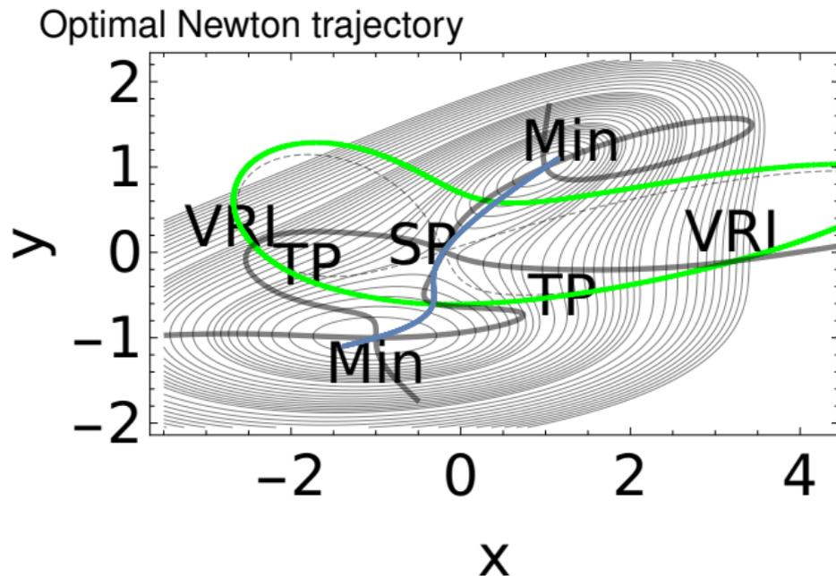
A special regular NT (blue) and a Gradient Extremal (thick black) cross the green line at the same point. This point is the BBP with lowest  $|\mathbf{g}|$  with respect to the others NTs crossing the green line. The regular NT indicates the optimal pulling direction.
