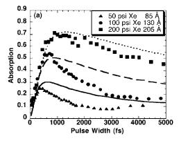
**Figure 3.** Absorption as a function of pulse length for different gas pressures, i.e. different cluster sizes (from Zweiback *et al* (1999)). The average cluster radii are 85, 130 and 205 Å, respectively. Solid lines are the results of calculations based on a nano-plasma model; see section 3.4.
