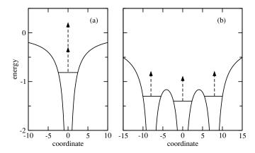
**Figure 5.** Schematic picture of the (inner) ionization process (a) in a single ion (e.g. Xe<sup>+</sup>) and (b) in a simple cluster of three ions (from Siedschlag and Rost (2004)). While it takes two photons to ionize the single ion, one photon is sufficient to achieve inner ionization in the case of the cluster.
