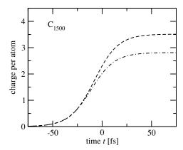
**Figure 16.** Time evolution of charge per atom for a C<sub>1500</sub> cluster in a Gaussian pulse at 12 keV with 50 fs pulse length for two different model calculations with (dashed line) and without (dot-dashed line) electron-impact ionization. After Jurek *et al* (2004a).
