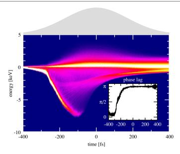
**Figure 9.** Time-resolved energy spectrum of cluster electrons under a laser pulse of the form  $F(t) = \exp(-\log 2(2t/T)^2)\cos \omega t$  with half width (pulse length) T = 400 fs and for a cluster of 9093 xenon atoms. Bright colour corresponds to a large number of electrons. The laser pulse envelope is indicated in grey. The inset shows the phase lag of the electronic CM motion, cf figure 7(d).
