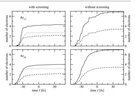
**Figure 13.** Number of created electrons (by photoionization: dashed line; by photoionization and subsequent decays: solid line; by intra-cluster tunnelling: dotted line) as a function of time t for two cluster sizes  $Ar_{13}$  (upper row) and  $Ar_{55}$  (lower row). We compare full calculations (left column) with those where screening, i.e. intra-cluster tunnelling, was excluded (right column). The laser field strength is  $\mathcal{E}=1$  au, other laser parameters as in figure 12.
