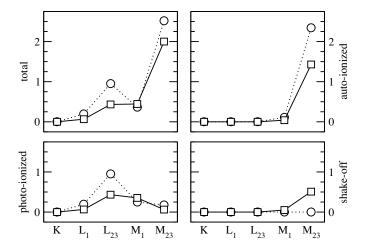
**Figure 14.** Number of electrons per atom for  $Ar_{55}$  due to photoionization, autoionization, shake-off process and their total sum with respect to the electronic shell they originated from. As in figure 13, full calculations including screening (square symbols) are compared to calculations excluding screening (circles).
