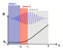
**Figure 1.** Sketch of cluster dynamics under a strong laser pulse in terms of the time-dependent cluster radius R(t). Atomic ionization (phase I), critical expansion (II) and relaxation (III); see text. The laser pulse is also indicated.
