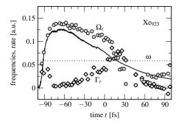
**Figure 8.** Parameters of the harmonic oscillator model (32) as calculated from the  $Xe_{923}$  dynamics in figure 7. Shown are the eigenfrequency  $\Omega_t$  according to equation (30) as a solid line and from equation (33) with circles, as well as the damping rate  $\Gamma_t$  from equation (33) with diamonds and the laser frequency (dotted line).
