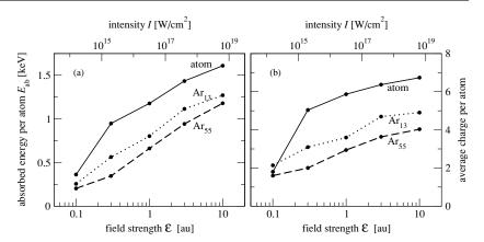
**Figure 12.** Absorbed energy  $E_{ab}$  per atom (a) and final average charge per atom (b) for two cluster sizes  $Ar_{13}$  and  $Ar_{55}$  produced by an XFEL pulse ( $\hbar\omega = 350$  eV, T = 100 fs) as a function of the field strength  $\mathcal{E}$  compared to atomic argon as a target. Each point is the average of ten simulations.
