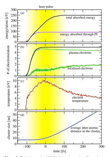
**Figure 3.** Typical scenario of VUV–cluster interaction. Dynamics of  $Ar_{147}$  exposed to a 20 eV FEL pulse with intensity  $I = 7 \times 10^{13}$  W cm<sup>-2</sup> and duration T = 100 fs, which is marked by the yellow/light-grey shaded area. From top to bottom: (a) total absorbed energy and energy absorbed through PI, (b) total electron number, number of plasma and transiently localized electrons, (c) electron temperature and (d) cluster size. Data from Georgescu *et al* (2007b).
