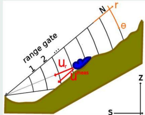
pulsed Doppler radar measurements
